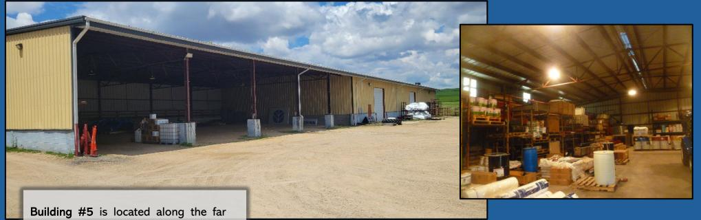
western edge of the property. It is a storage type building. This building is unheated, and the southern portion of the building is a 3-sided shed building section, being open toward the east. This is a pre-engineered steel building with metal siding. There is 9,600 square feet of enclosed warehouse area, plus 6,000 square feet of three-sided shed area. The warehouse area has concrete flooring, while the three-sided shed area has gravel floors. Building height is about 14 feet.
